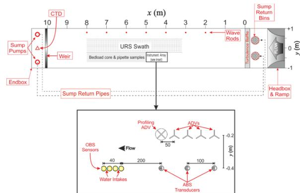
Fig.3. Instruments settings in the experimental flume channel
