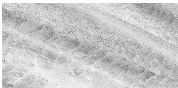
Figure 1. Side scan sonar images from the Jade area (Germany). Individual (starving) megaripples are separated by large gaps in which underlying glacial till and coarse sediment shows a high backscatter due to a lack of sediment. In an area at 10 nm distance with sufficient sediment supply this is not observed.
