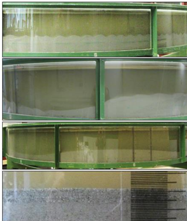
Figure 6 – Examples of bedforms that developed during the experiments. Sediment mobility increases from top (ripples) to bottom (upper plane bed).
