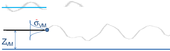
Figure 4. Vertical ship motion above horizontal bottom
