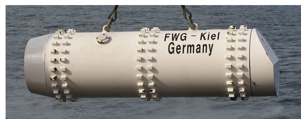
Figure 2. BRM, length: 1.70m, diameter: 47cm, weight: 5.0 kg. Bow ring at the right side (Wever et al. 2004).
