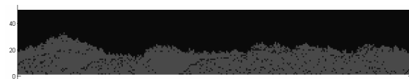
Figure 3. The sorting mechanism leads to veneers of coarse (black) material underneath the mobile fines (gray).
