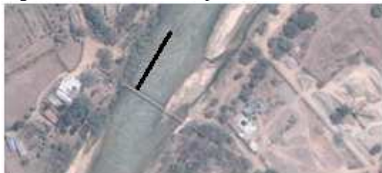
Figure : September 2007, we count 11 sand waves on 76 m, thus \lambda_{bf} = 6.9\text{m} . Source: Google earth®.
