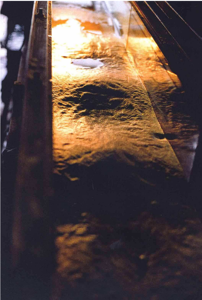
Figure 3. Oblique view of 3D antidunes after draining. The width of the flume is 30 cm. The flow was along a direction away from the viewer. Gently undulated, 3D, round hummocks and swales are prominent. The wavelength and wave height of the antidunes is approximately 50 cm and 2 cm, respectively. This is the case for n = 1 .
