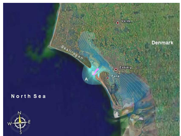
Figure 1 Computational grids of the morphodynamic model of the Grådyb tidal channel. A denotes the coarse overall grid, B the higher resolved detail grid.
