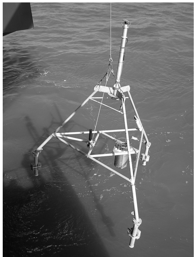
Figure 7. Scanning sonar tower during deployment. The total height to the rotary sonar is 4.5 m. The power supply and recording electronics are in the container near the centre of the stabilizing construction, two current meters can be seen on the far right leg and near the centre of the stabilizing construction. For improved stability lead weights were attached to the vertical legs of the tower.
