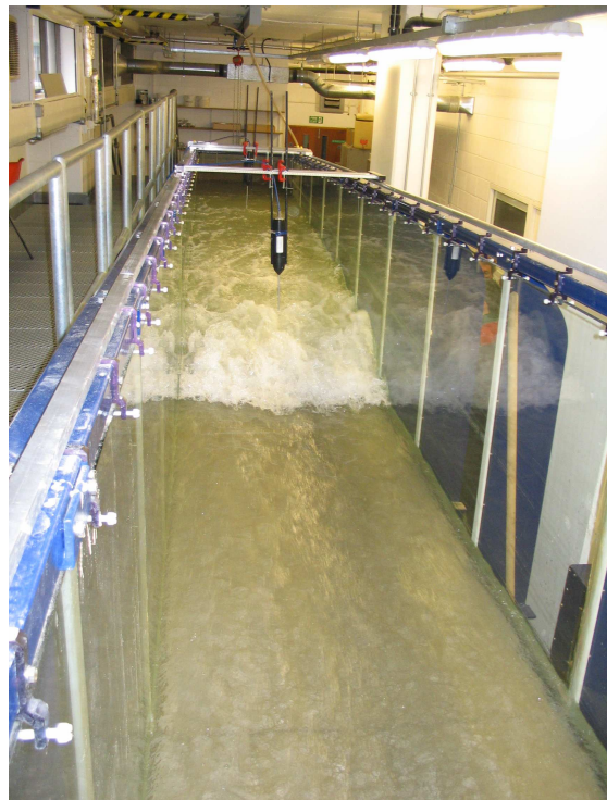
Figure 2. View downstream over a hydraulic jump in the ENV flume. Flume width is 1m.
