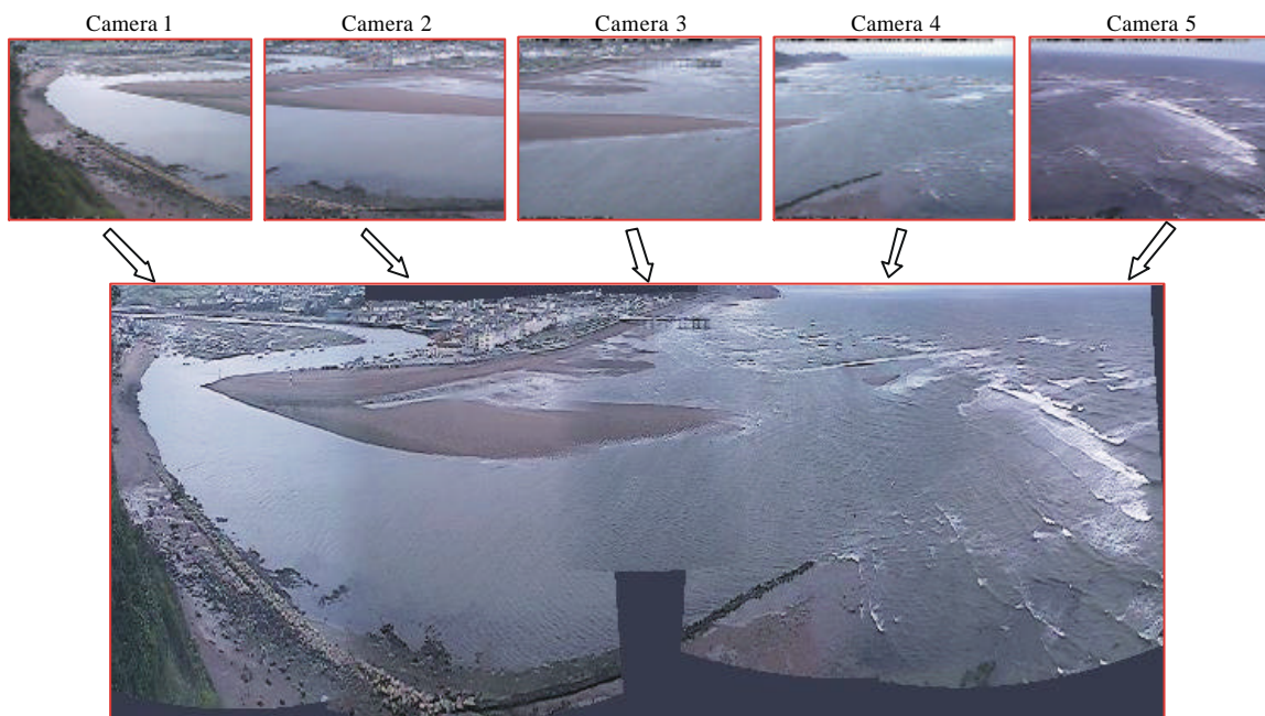
Figure 2: Views from the individual five cameras in the top, merged in the bottom at low-tide (17 May 1999, 14:00).
